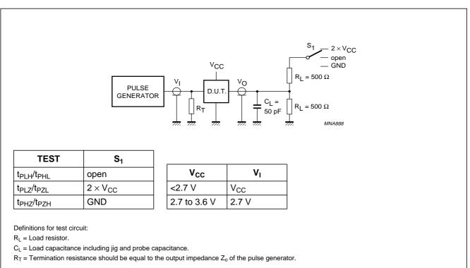
Fig.12 Load circuitry for switching times.
